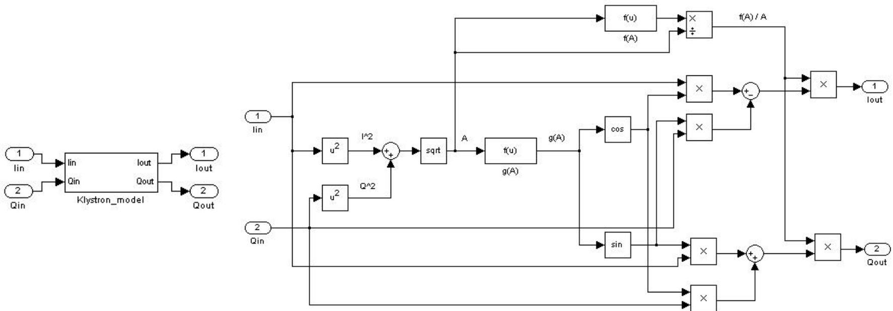
The model of the klystron in Simulink
