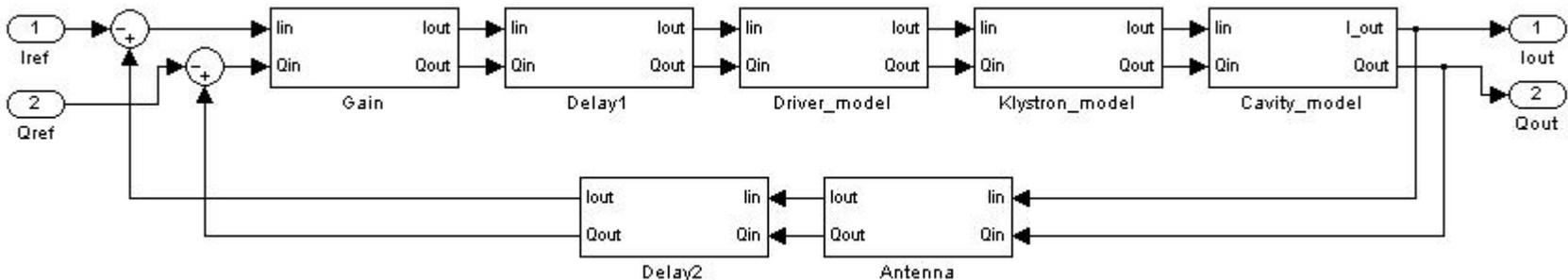
The simulation model of the cavity controller
