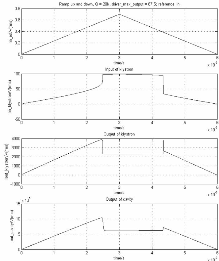
The ramp responses of the model with a clamped and overdriven klystron
