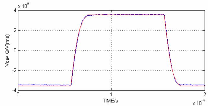
Measured (blue) and simulated (red) step responses in the cases of the inverted and non-inverted phase shift of the klystron
