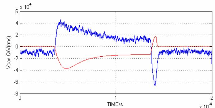
Measured (blue) and simulated (red) step responses in the cases of the inverted and non-inverted phase shift of the klystron
