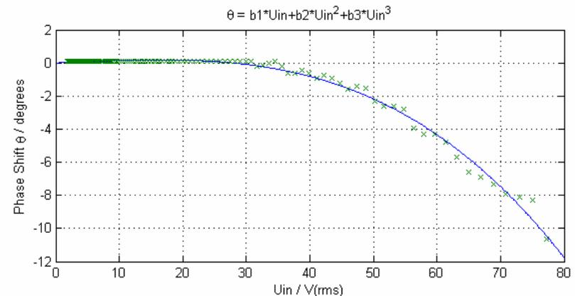
AM-AM and AM-PM curves of a klystron
