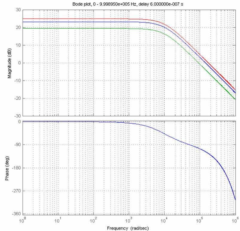
The Nyquist and Bode plots of the open loop model with three values of gain
