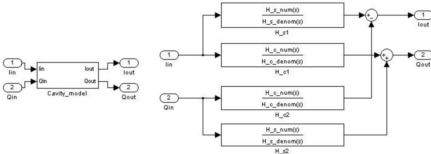
The model of the cavity in Simulink
