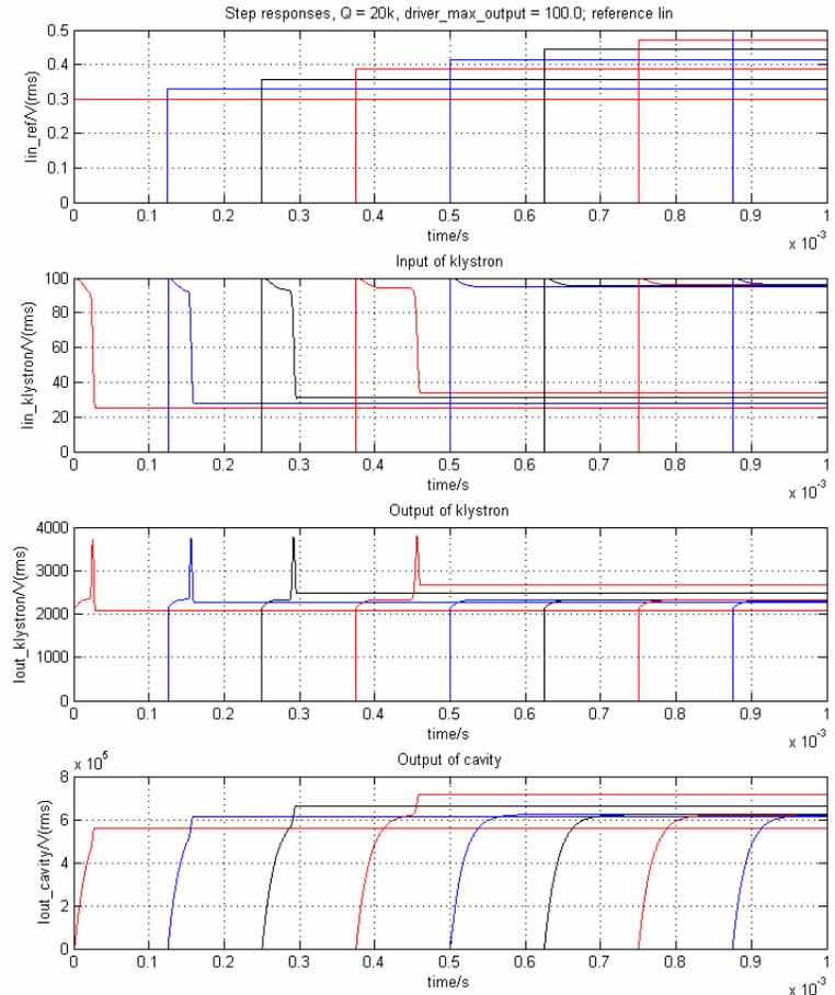
The series of step responses of the model with a clamped and overdriven klystron
