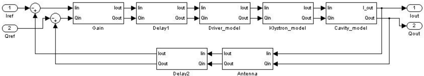
The simulation model of the cavity controller
