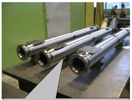
3 vacuum tanks were manufactured at the "Raduga" Plant (Dubna) in cooperation with Izhevsk in 2002. The pre-production unit (2 vacuum tanks) was tested at CERN in 2003 and revealed welding quality issues that are being resolved (1 tank leaking, both tanks rejected by LHC-VAC)
