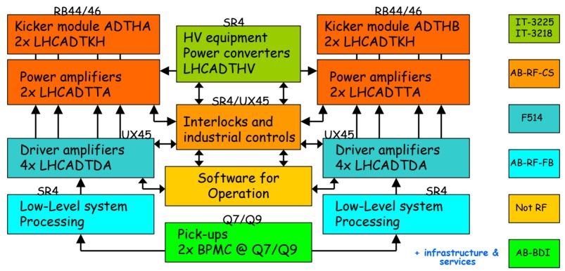
Shown is one "system". There are four independent systems, one per plane (H/V) and beam.
