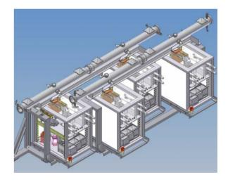
Situation in tunnel in Summer 2003, view from UX45 along LHC tunnel Damper equipment (two modules with two kickers each per beam and their power amplifiers)
